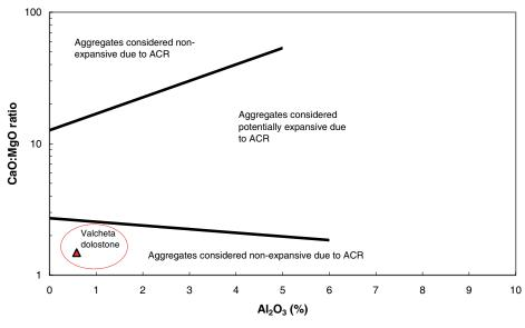
FIGURE 1. Result of CSA A23.2-26A chemical test
