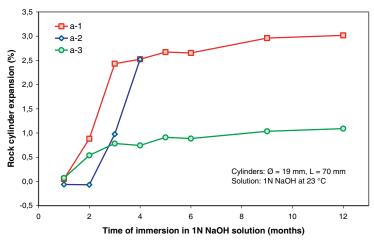
FIGURE 2. Expansion of rock cylinders in 1N NaOH solution
