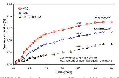
FIGURE 4. Expansion of concrete prisms (VD-c) using LAC or HAC + FA (CPT)
